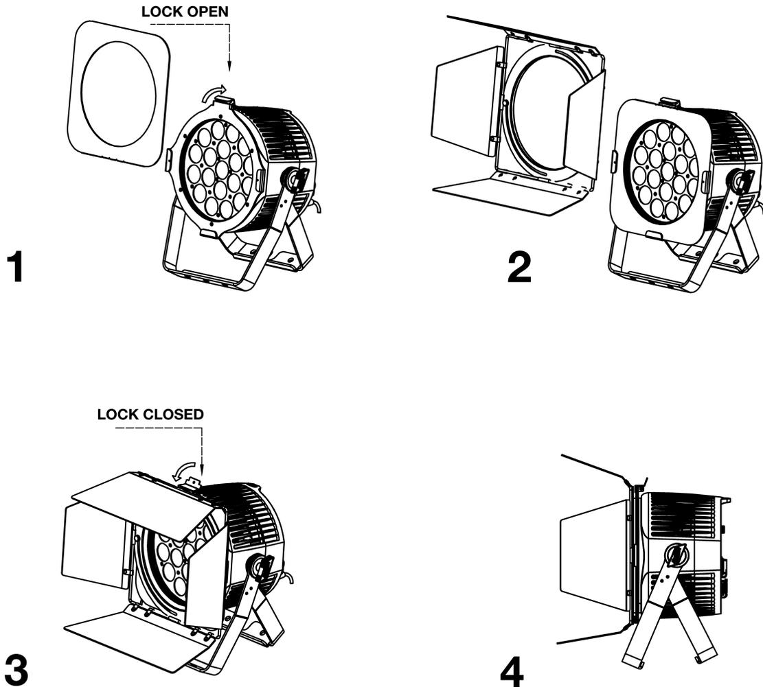
1. Attach **Gel Frame Holder / Screw Kit** to fixture, tightening each screw by hand.
